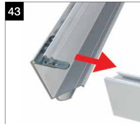
Fix cleats into the small return cornice mid sections and offer up to the cornice section fitted previously fixing with CHA007.
