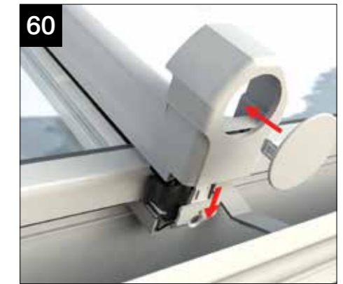
Fit the glazing bar end caps by sliding onto the end of the bars using the fixing blocks. Push fit the insert into the end cap.
