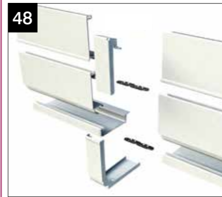
Whilst ensuring that the joint remains located in position, screw fix using self drilling screws 8PSR42-25BLK. Slide the bracket into place ensuring bracket cleats slot into the top cornice section and screw fix using CHA007. This is done similar to the corners shown previously.
