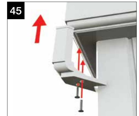
Whilst ensuring that the corner remains located in position, screw fix using self drilling screws 8PSR42-25BLK.
