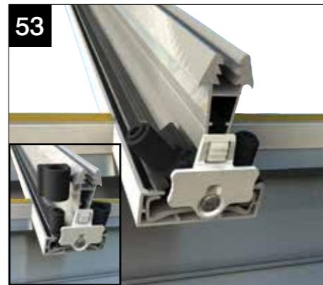
Snap off appropriate handed glazing stop. Handing marked on base of moulding. Line up the rounded edge on base plate next to central web of glazing bar then tuck neatly under gasket side of bar. Rotate moulding into position. Push the grommet over the post as shown.
