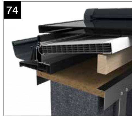
74 Sit modesty panel inbetween the bars of the glazed section and on the shelf of the eaves beam. Position the previously constructed frame so that it lifts the front panel and supports it.
