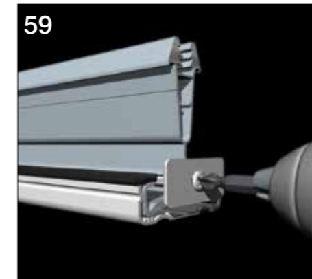
At the lower eaves end fix the glazing bar end cap brackets onto the end of the bars using fixing EFSA021.
