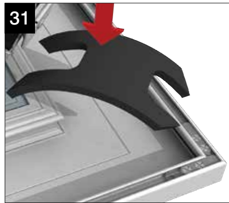
Apply sealant to the foam sealer strips and foam 'H' component. Position foam components into the lower cornice section and press down.
