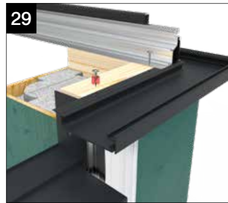
Fix the small cornice returns to the columns through the pre-drilled holes using fixing NRTF050.
