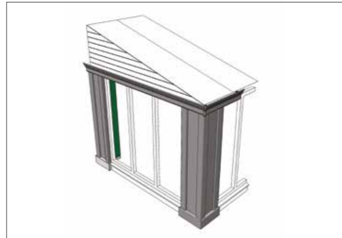
Self manufactured firring with abutment. This design uses Ultraframe's Gable support beam - see illustration B on p31
