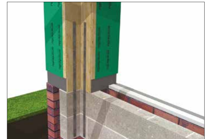
LARGE 90° CORNER Fasten straps down inside of walls of large 90° corner column
