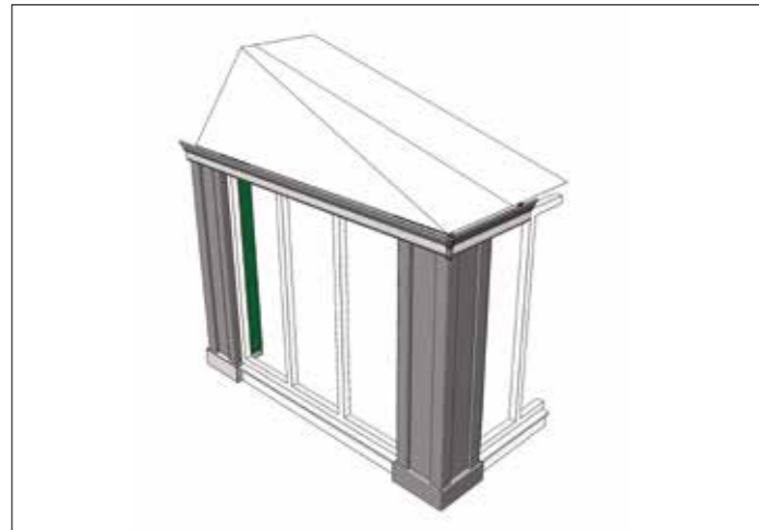
Hipped end with abutment
