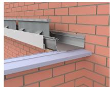
When using the reinforced box gutter, it MUST be supported at each end by either hup walling, a brick pier, or a post (by 100mm minimum). When the overall length is greater than 6m and a split is required, the box gutter MUST be supported by at least 100mm either side of the joint.
